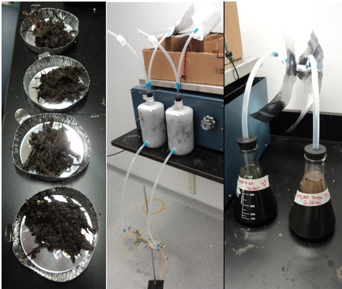
Figure 1: Samples taken from the mixtures for the first bench-scale reactors (left); bench-scale reactors, one with P&P AD sludge and one without, gas bags on the top and IV bags on the bottom for the purpose of manual leachate recirculation (center); blanks which have the same quantity of inocula as what was mixed into the reactors.
