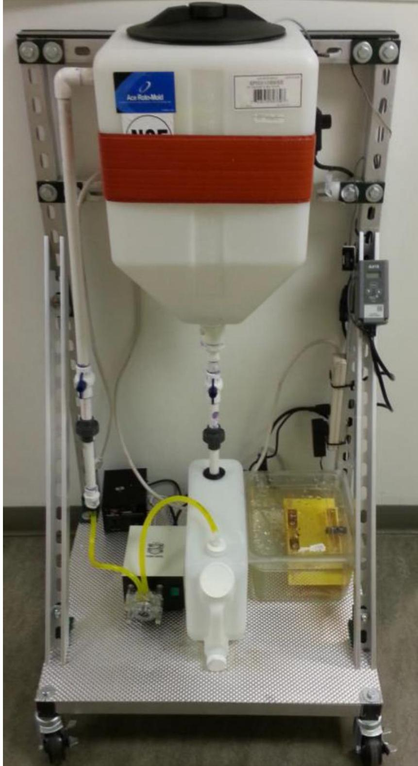
**Figure B2:** Photograph of fully-constructed 10-gallon pilot-scale HS-AD system.
